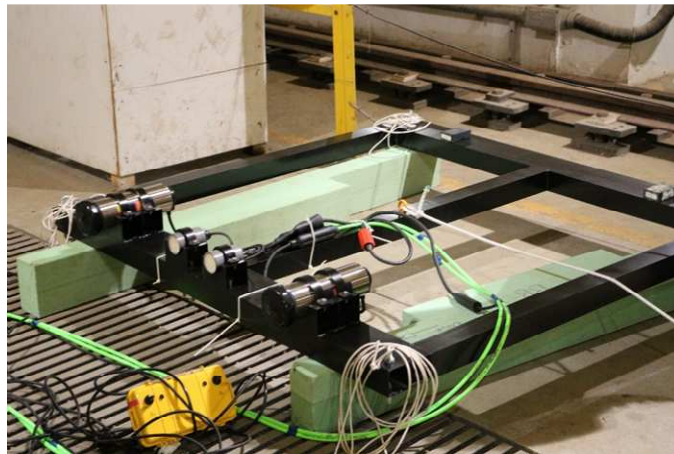
Figure 8 The support with the cameras and the illuminators attached
